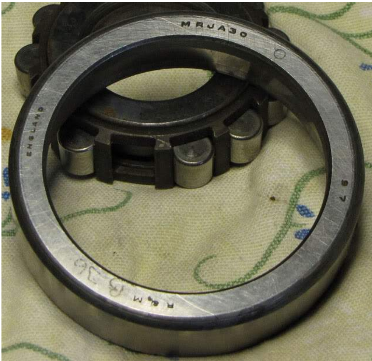
Illustration 26: R&M MRJA30 removed from a 1969 Commando (Access Norton Forum 'DogT')
