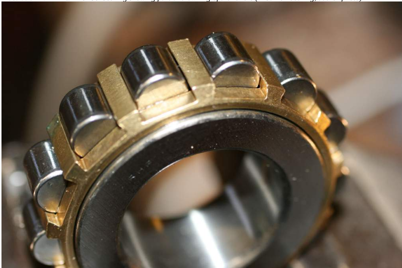
Illustration 4: RHP 6/MRJA30 'bearing showing partial crowning of the rollers (A Curzon bearing, author photo)
