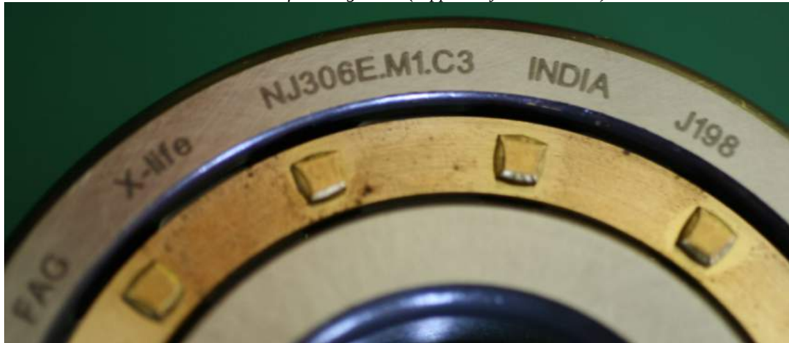
Illustration 17: FAG NJ306E Manufactured on 13/07/15, i.e. as marked 15071300
