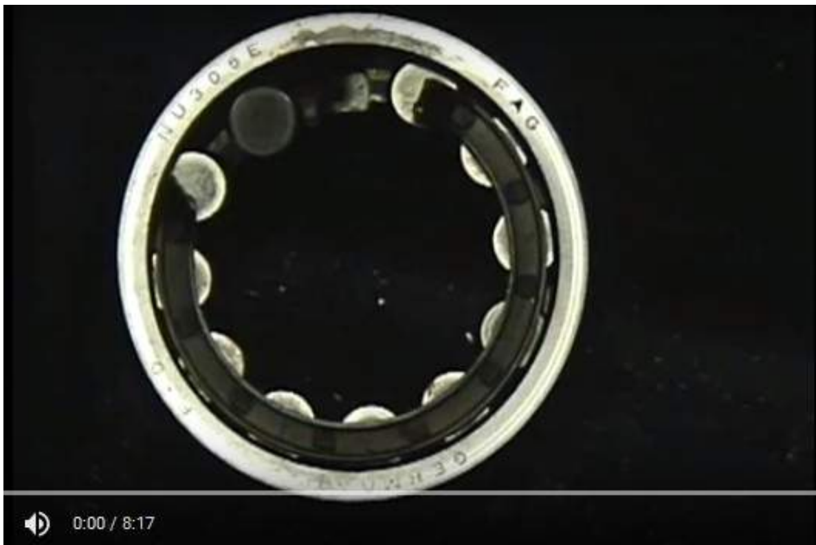
Illustration 12: FAG NJ/NU306E with roller removed for measuring (see Table 4, Page 15 for explanation of NJ & NU)
