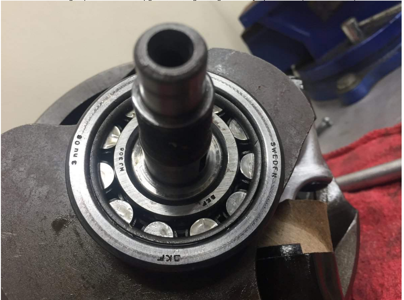
Illustration 31: Image of SKF NJ306 configured bearing. Image courtesy of Brian4.2 (Access Norton).
